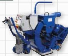
The AC inverted drive-motor for self-propelled operation features an integrated brake which helps maintain speed on ramps and inclines. This improves productivity and promotes a more even and consistent blast pattern and surface profile. Attached to the 8-54DC or other suitable Blastrac dust collector, it operates virtually dust-free. A slide-out screen in the shot hopper facilitates the removal of large debris.
