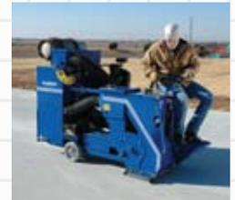
The Blastrac 1-10DLP is a mid-range system ideal for applications such as industrialized plant and warehouse floors, parking garages, bridges, highways, airport runways and ship decks.
