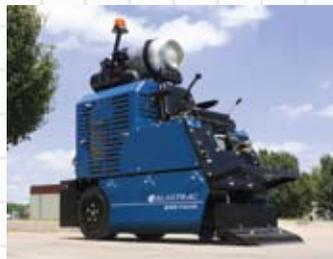
Maximum torque is produced through the 42 hp Hyundai engine giving the BMS-T4200 the power that is needed for the most grueling and time consuming floor removal jobs. Exhaust scrubbers reduce emissions to meet or exceed CARB and EPA requirements. The precision hydraulic steering gives the operator optimum control in maneuvering, and an auxiliary hydraulic system can power hydraulic attachments such as diamond grinders or rotary cutters.
